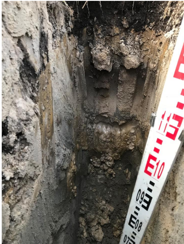
TP9 encountered 0.25m of topsoil overlying firm clay to 0.55m, overlying sand. Groundwater was encountered at 0.7m.
