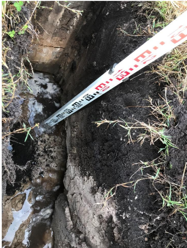
TP2 encountered 0.25m of topsoil overlying sand. Groundwater was encountered at 0.9m.
