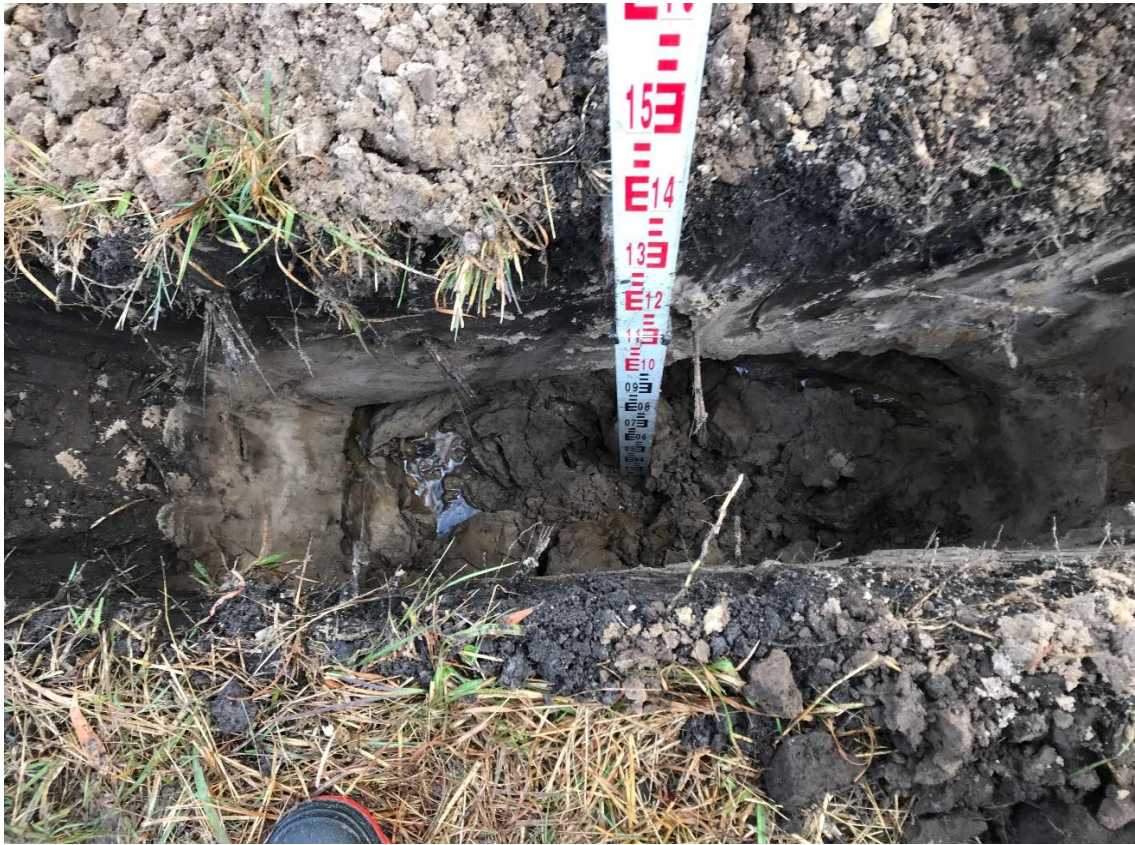
TP7 encountered 0.25m of topsoil overlying sand. Groundwater was encountered at 1m.
