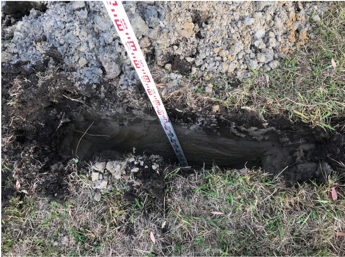
TP8 encountered 0.15m of topsoil overlying firm clay to 0.35m, overlying sand. Groundwater was encountered at 0.95m.
