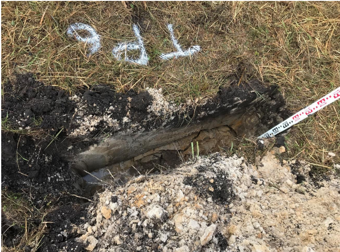
TP6 encountered 0.2m of topsoil overlying sand. Groundwater was encountered at 0.8m.
