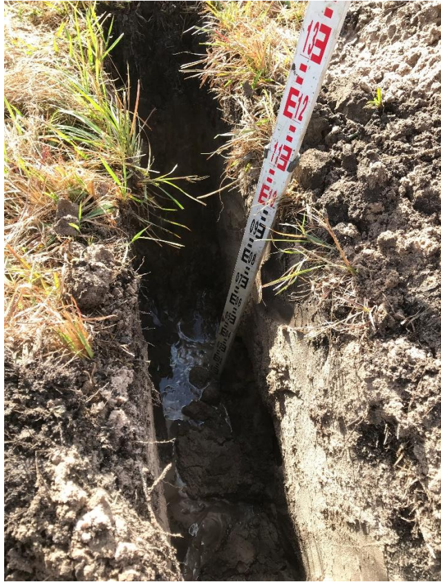
TP1 encountered 0.2m of topsoil overlying sand. Groundwater was encountered at 0.7m.
