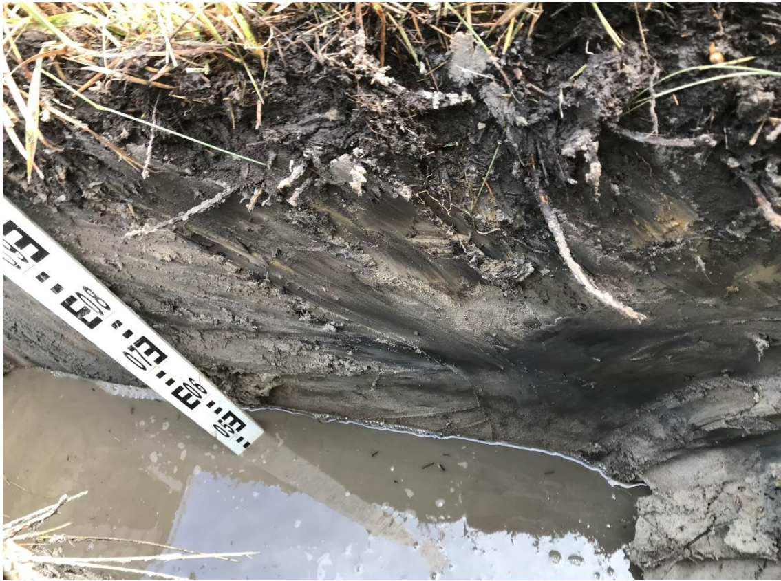
TP3 encountered 0.1m of topsoil overlying firm clay to 0.4m, overlying sand. Groundwater was encountered at 0.7m.
