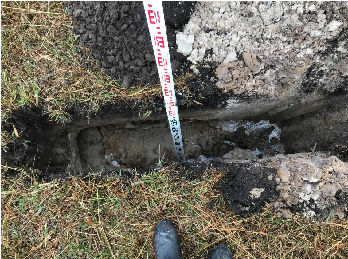
TP5 encountered 0.25m of topsoil overlying sand. Groundwater was encountered at 0.9m.
