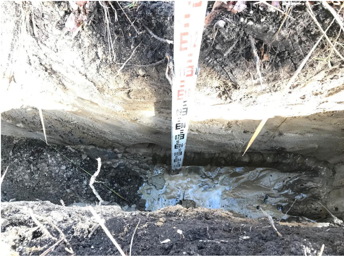
TP11 encountered 0.2m of topsoil overlying sand. Groundwater was encountered at 0.8m.
