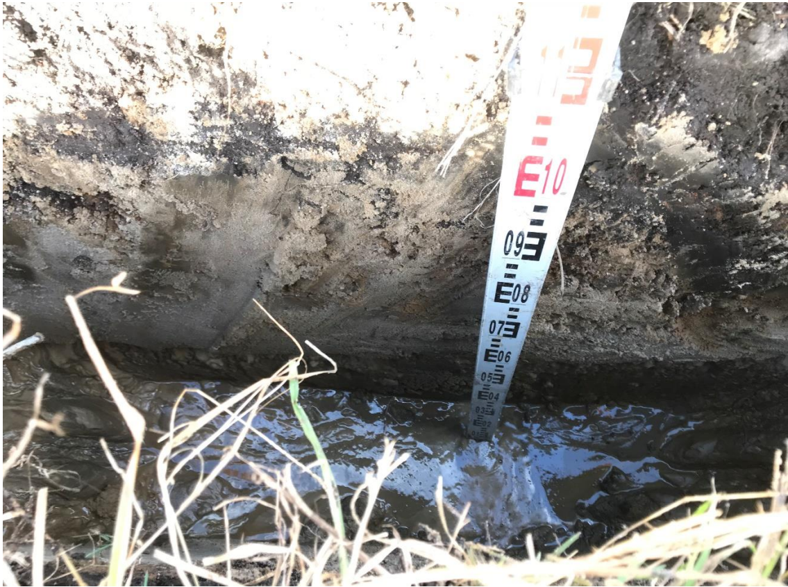
TP4 encountered 0.2m of topsoil overlying firm clay to 0.4m, overlying sand. Groundwater was encountered at 0.65m.
